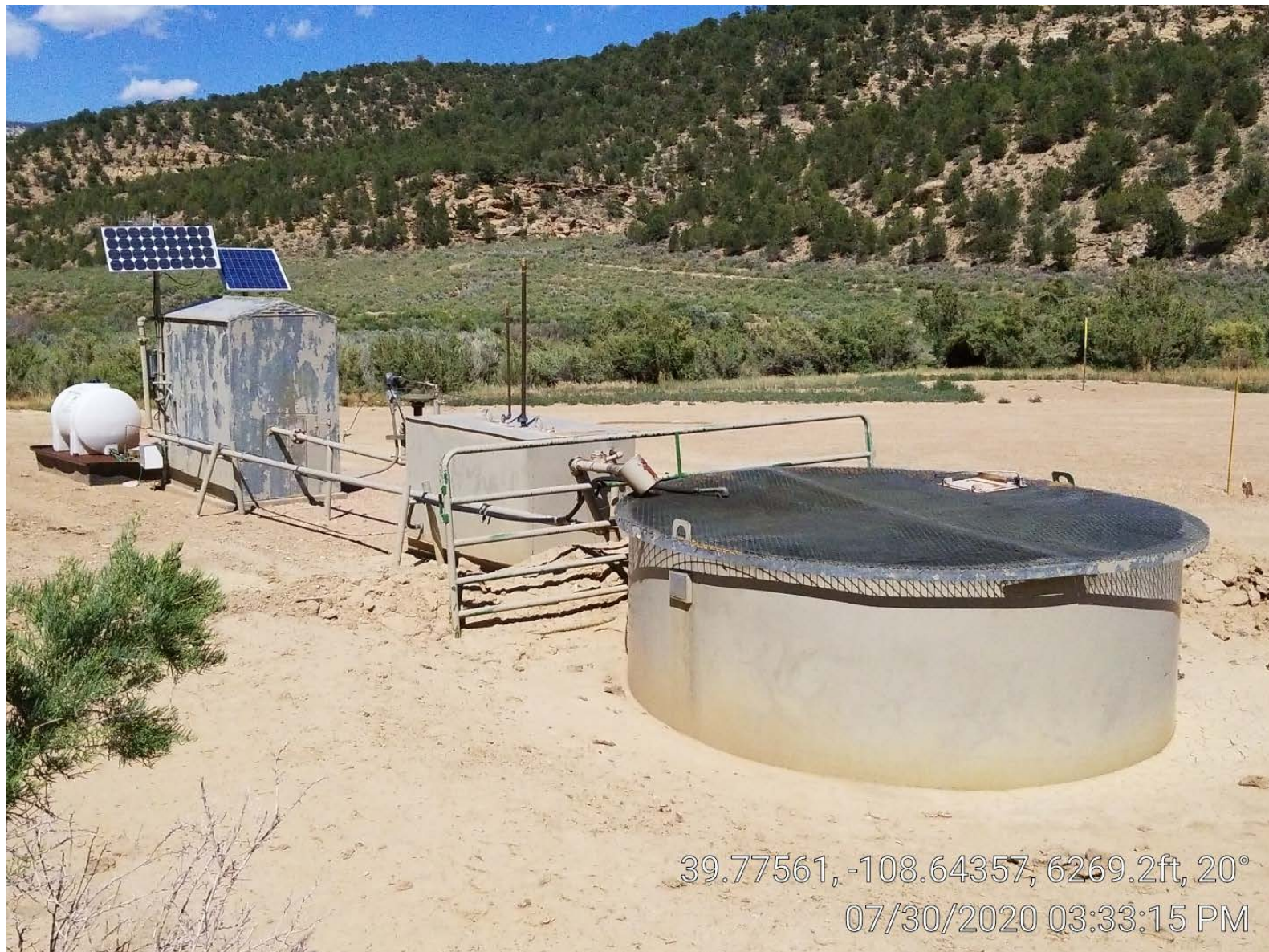
Photo 3. Meter building, separator, tank.
