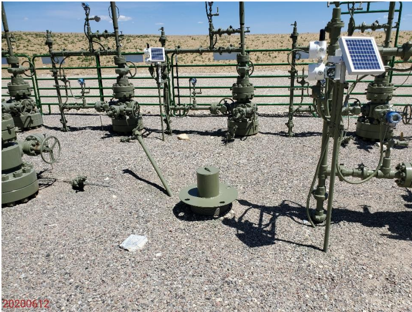
Photo 5: Photo of what appears to be the capped 045-23206 well. There does not appear to be signage for this well.
