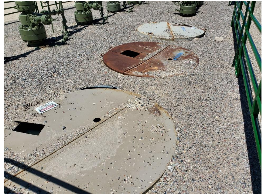
Photo 6: Photo of what appears to be 3 conductor settings for wells on the Location. There does not appear to be signage associated with these conductor settings/wells.
