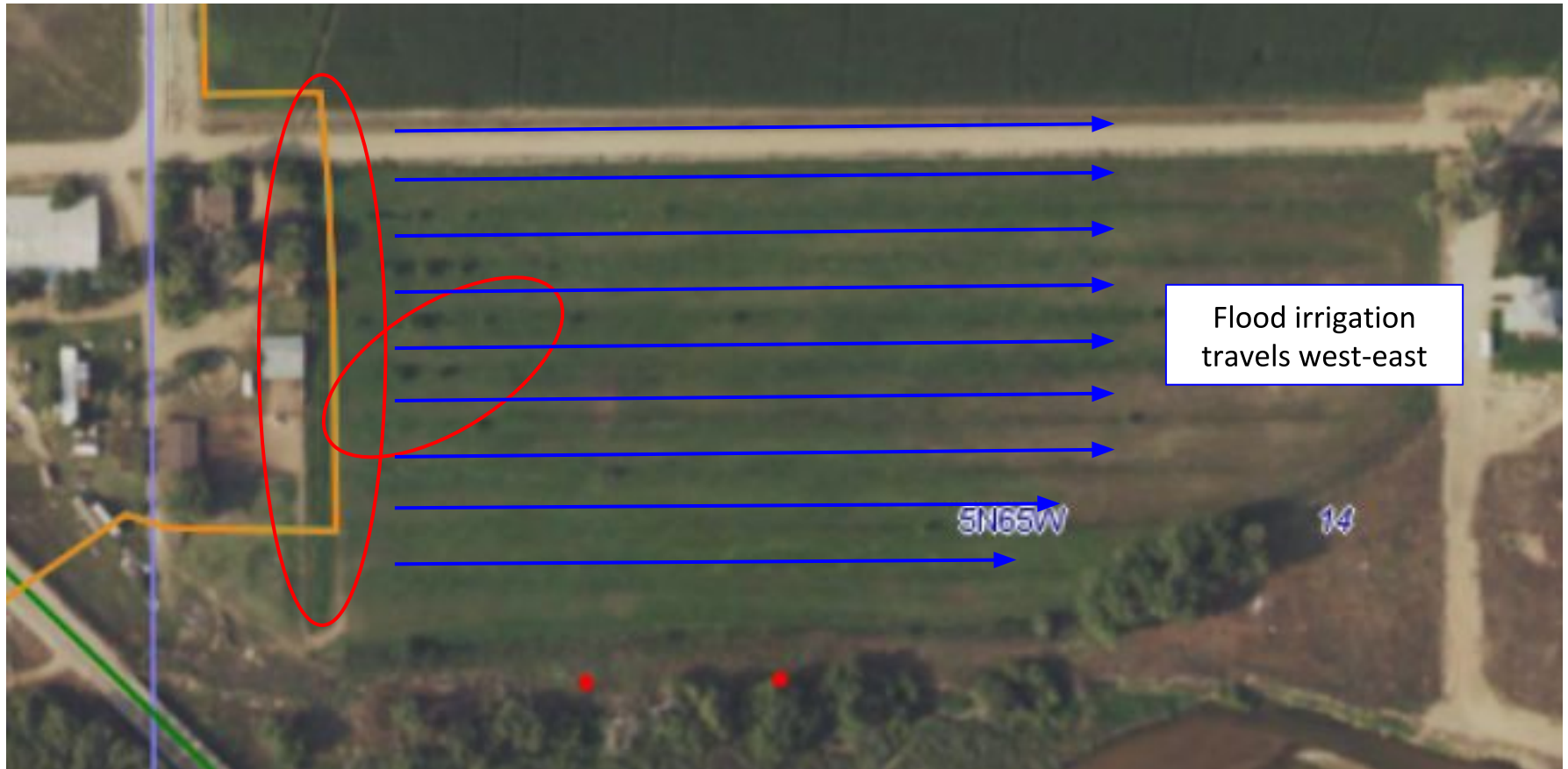
Photo 1. COGCC COGIS 2017 aerial imagery illustrates approximate areas concerning a complaint filed by the surface owner. An active crude oil line (orange line) was first installed and then a second line (gas) was installed later. The second line is associated with the complaint issues.
