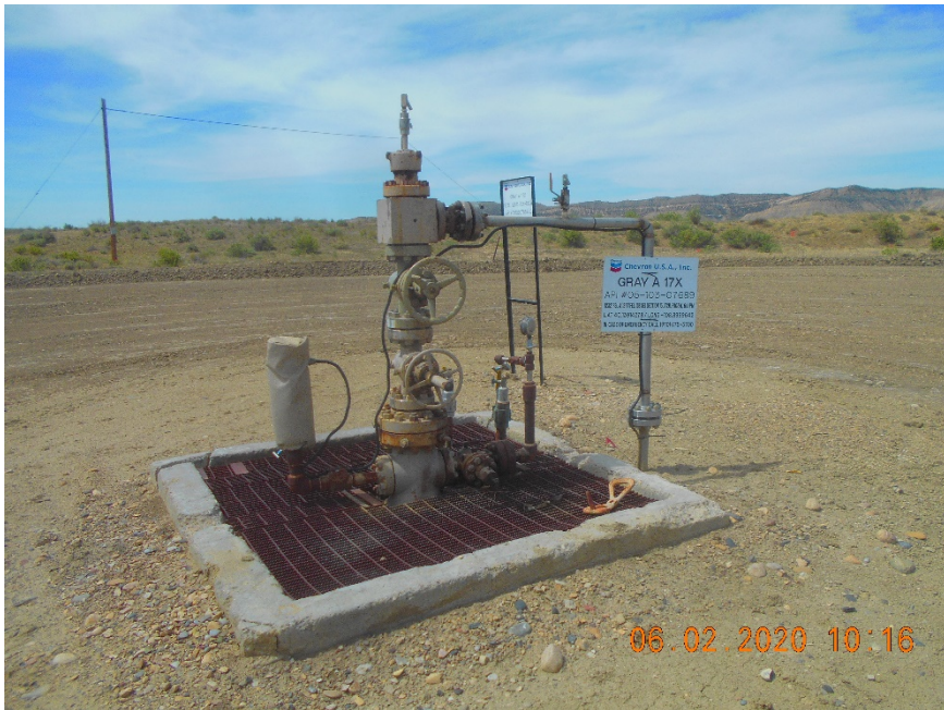
Injection wellhead
