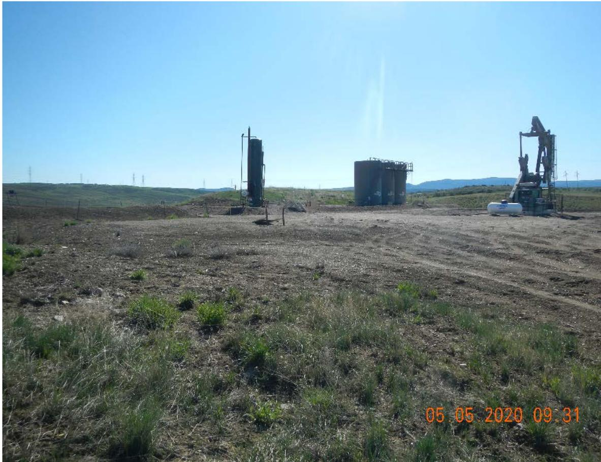
Photo #5 Flare Pit to left of Photo (Note: berm).
