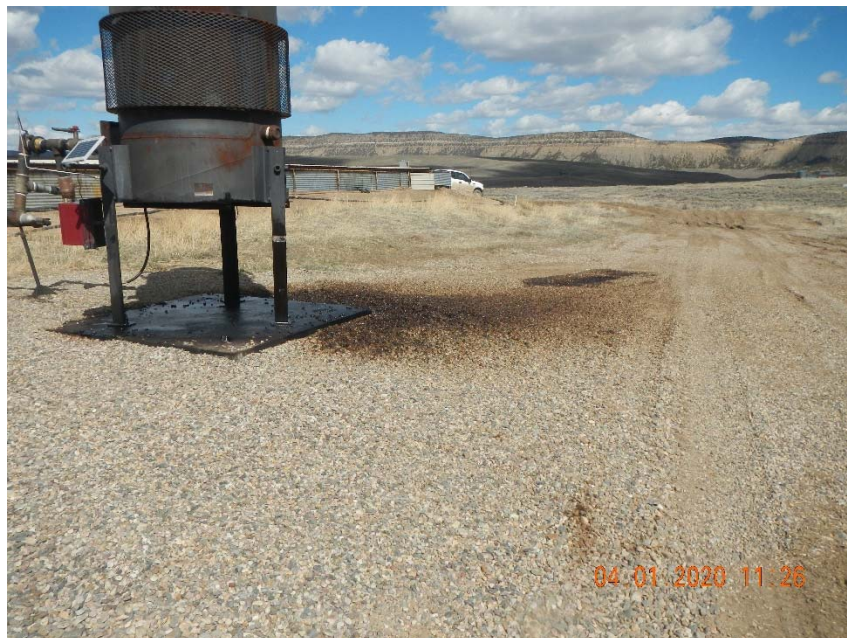
Photo 2. Stained soil under combustor.
