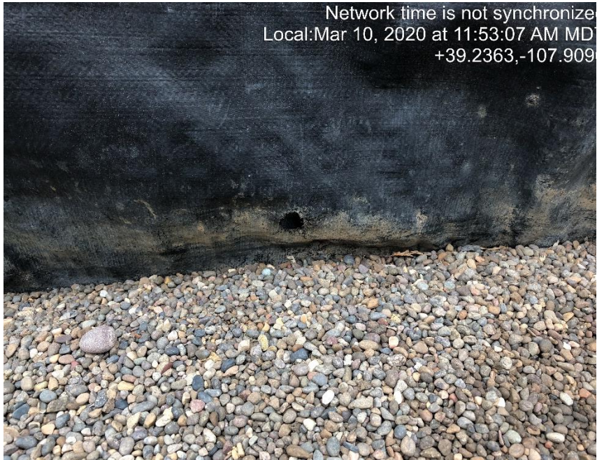
Photo #0736 Multiple holes through out tank containment liner.
