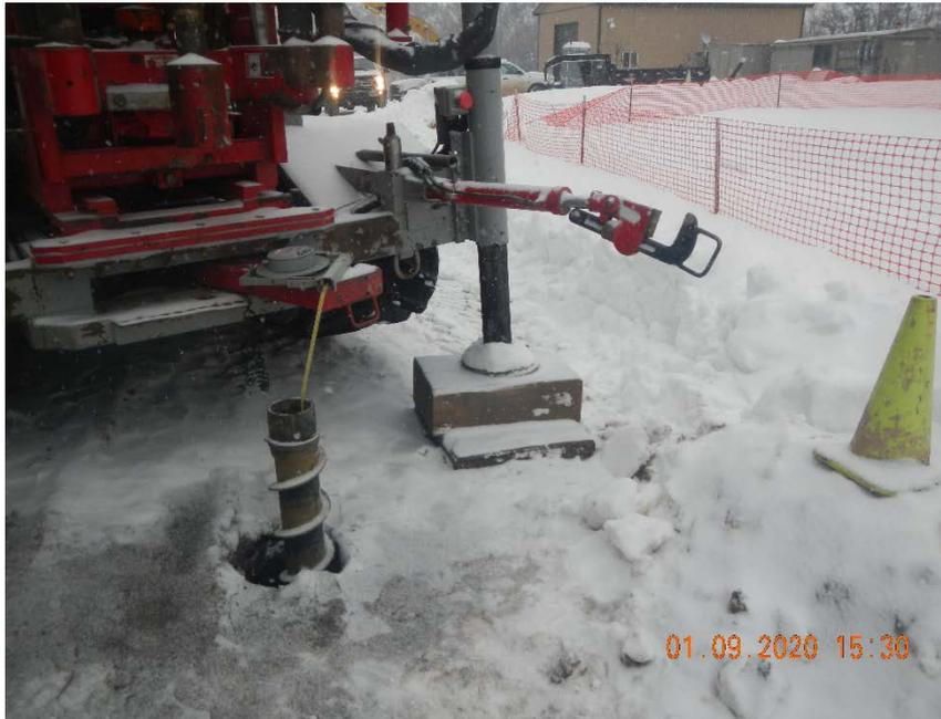
Photo #2 measuring groundwater depth on west side of old soil storage pit. Note: shop and pump building in background for reference.
