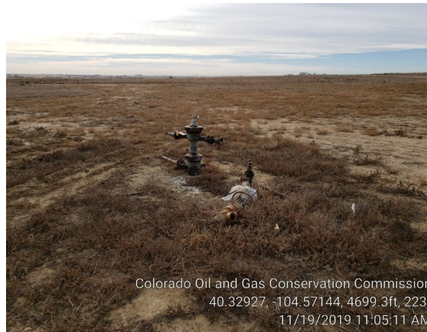
Photo #2 Wellhead, No Well or Emergency contact information. On 11/19/19
