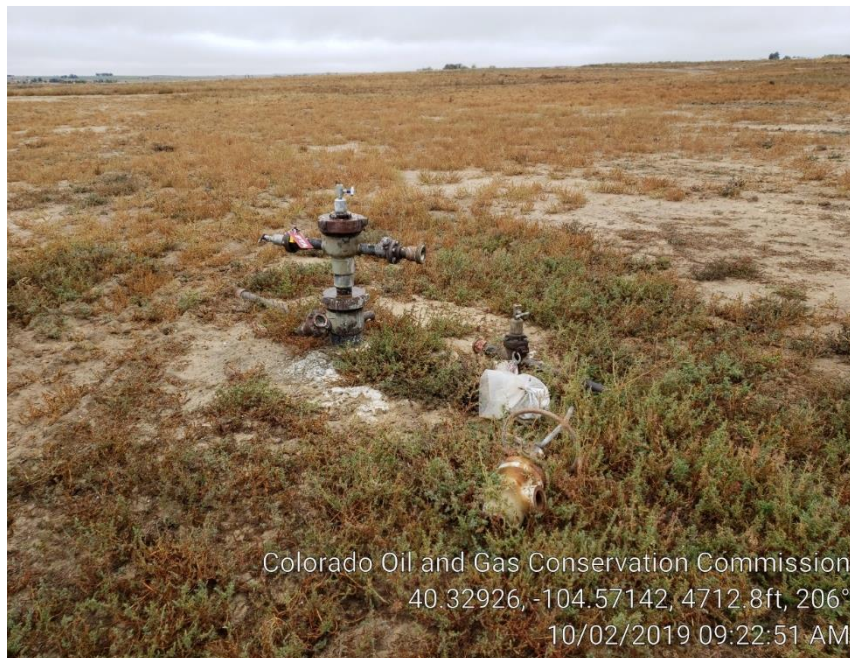
Photo #1 Wellhead, No Well or Emergency contact information. On 10/2/19
