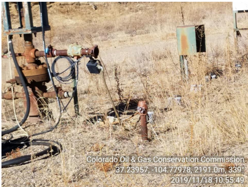
PHOTO 3: UNUSED RISER. REMOVE RISER OR PUT BACK IN USE AS PER NTO AND RULE 603.f. CA DATE 02-12-19
