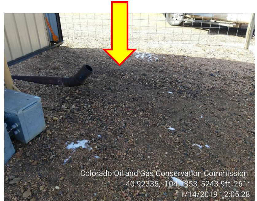
Photo 4 – Stained Soil at Exhaust
