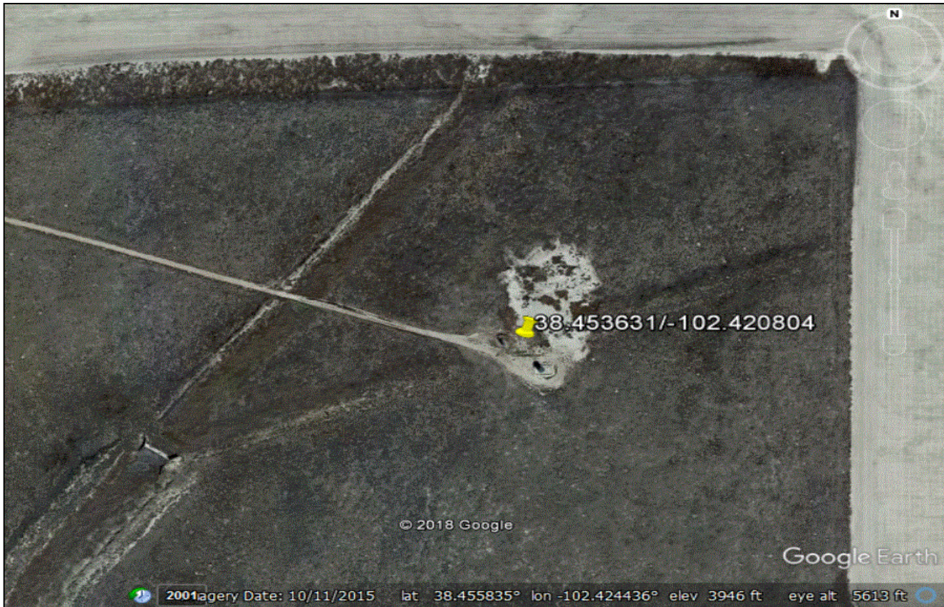
Photo 7. View of aerial image shows area north of the location bare of vegetation which may be the result of a former spill.
