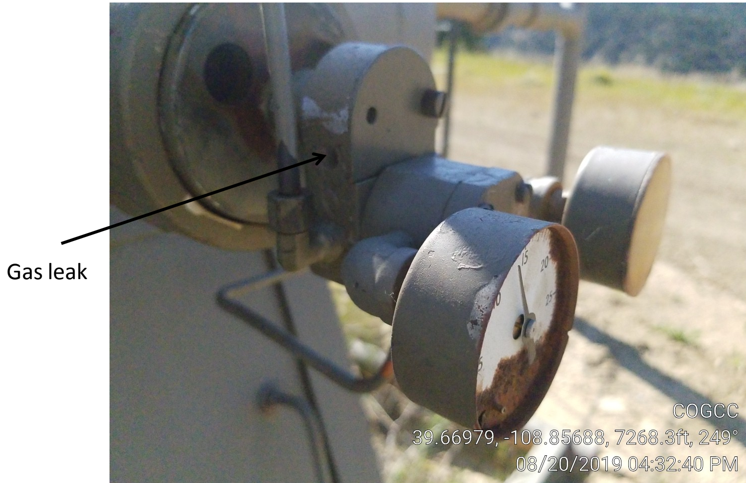
Photo 3. Separator gas leak.
