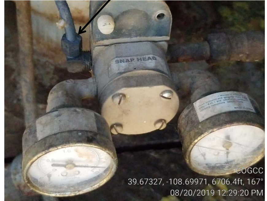
Photo 3. Separator leak.
