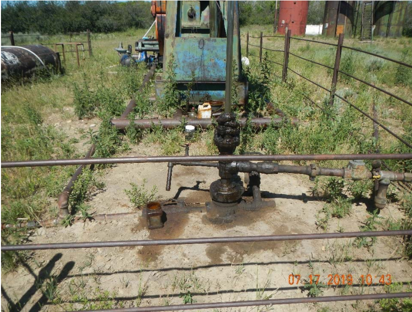
Photo 1. Stained soil at wellhead.
