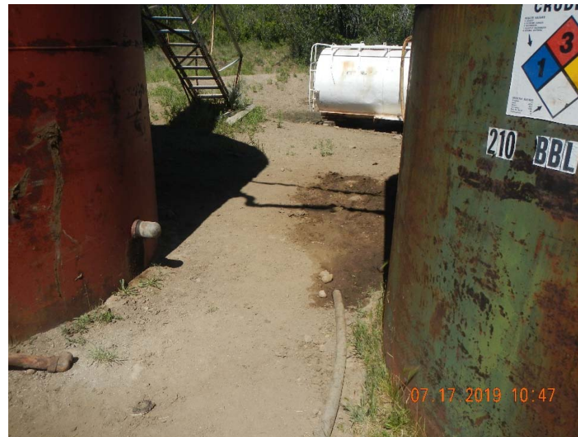
Photo 12. Stained soil in tank battery.
