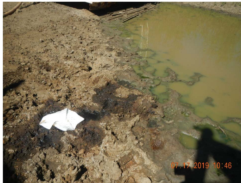
Photo 8. Stained soil and debris in tank battery.
