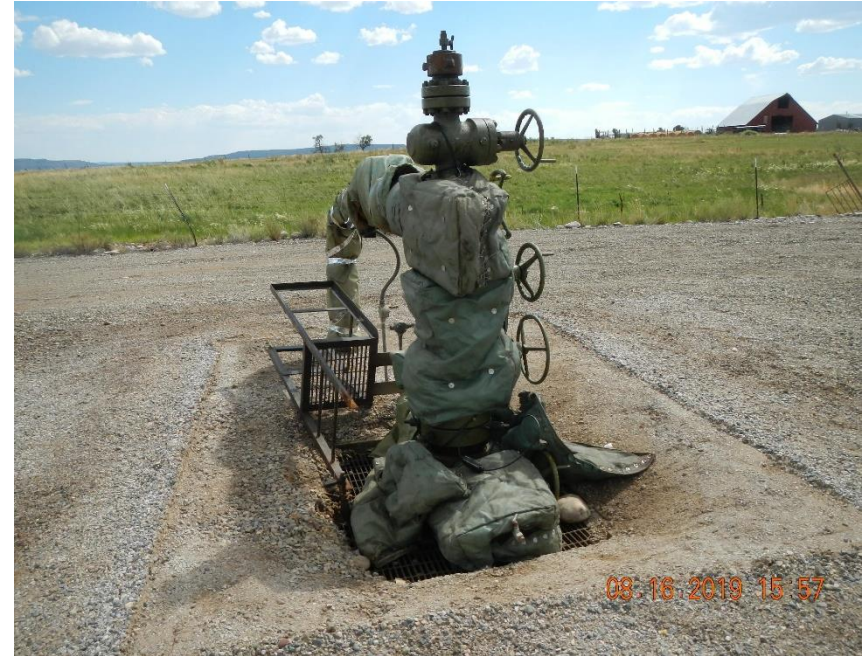
Luchini Water Disposal Well #1 with well house removed.
