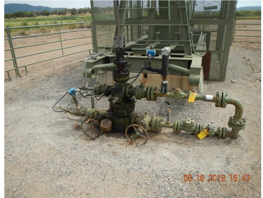
Stained and wet well head at the Luchini 32-6-12 #1.
