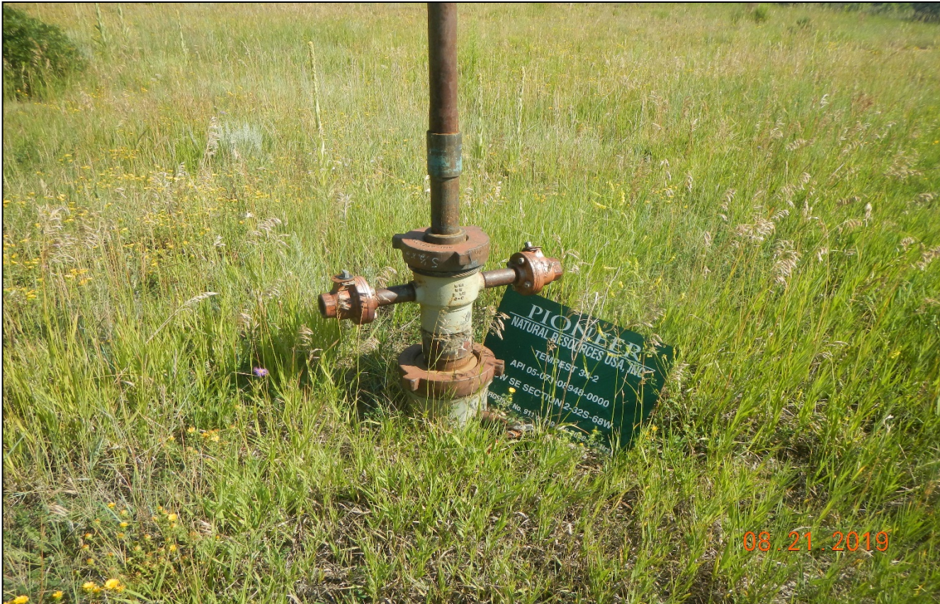
Photo 3. Well is temp abandoned. Well sign needs to be updated and securely fastened.
