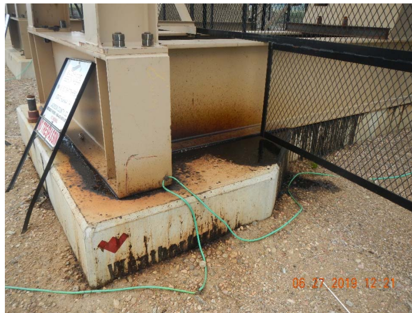
Photo 2. Stained soil and free product at pump jack.
