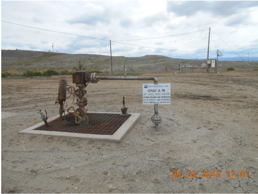
Injection wellhead
