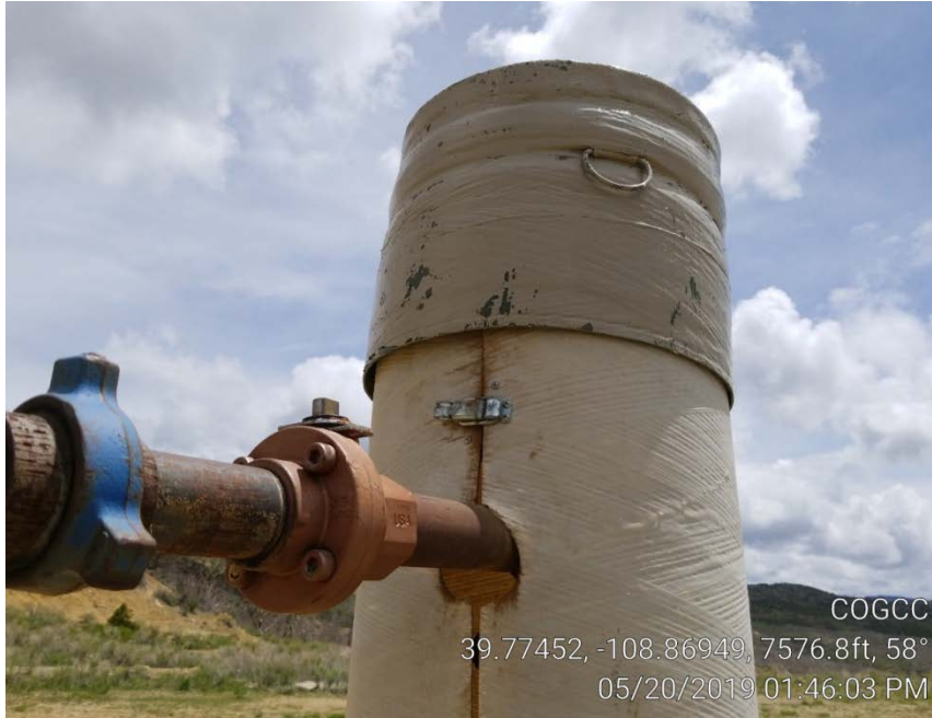
Photo 2. Gas leak in upper part of well head.
