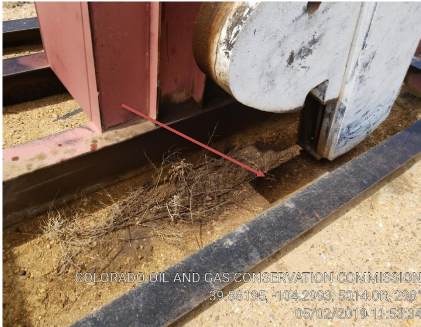
Pic 3 stained soil below counterweight.
