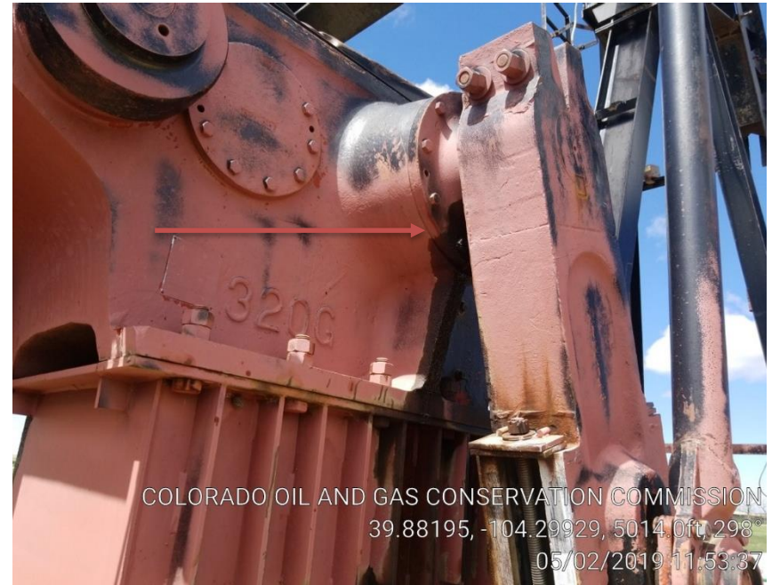
Pic 4 what appears to be a leak on pumping unit.
