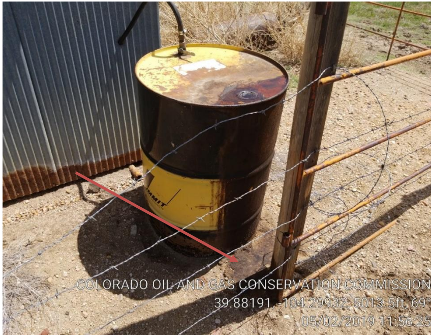
Pic 7 unknown barrel contents, no containment, appears to be leaking stained soil
