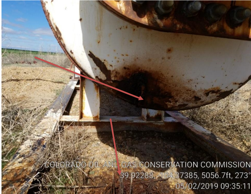
Pic 5 stained soil possible leak
