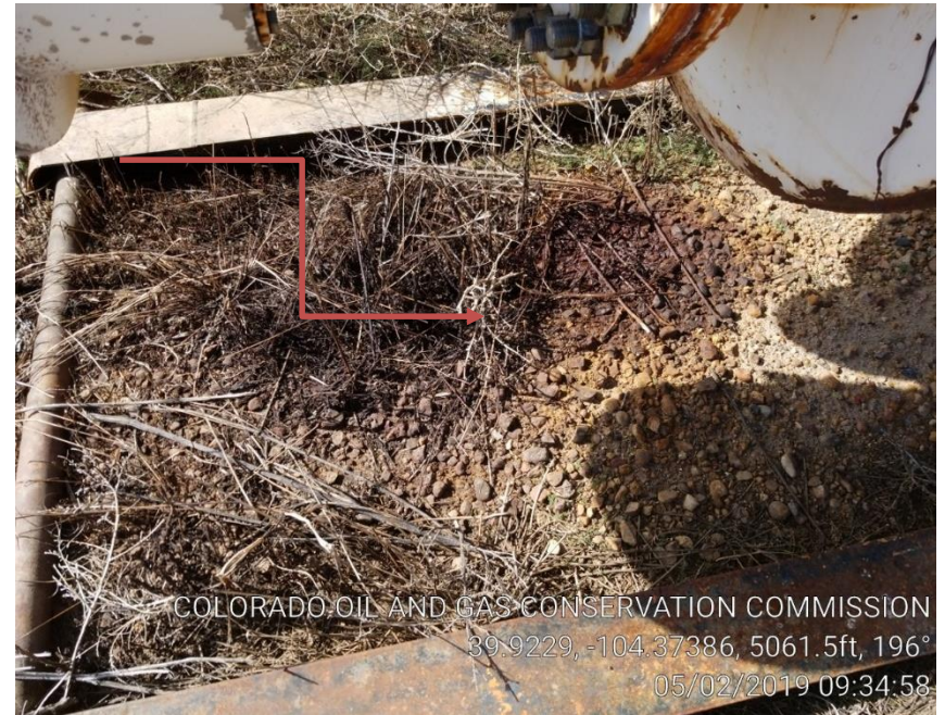
Pic 4 possible leak stained soil.
