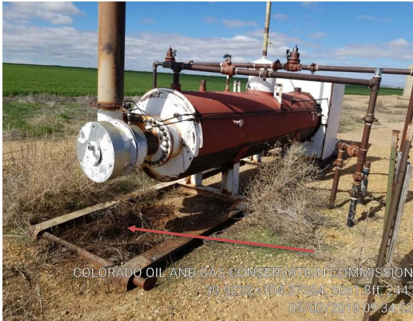
Pic 3. Separator possible leak. Stained soil
