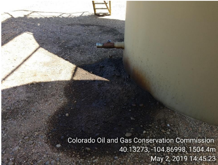
Photo 3 Stained soil around produced water tank
