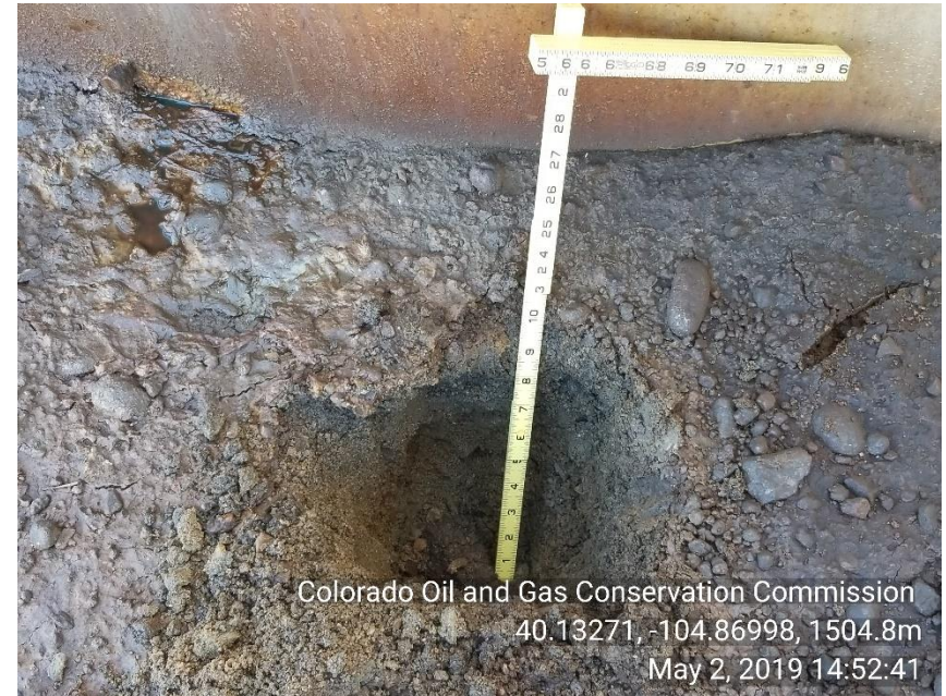
Photo 10 Dug down approx. 12 in ground still saturated.
