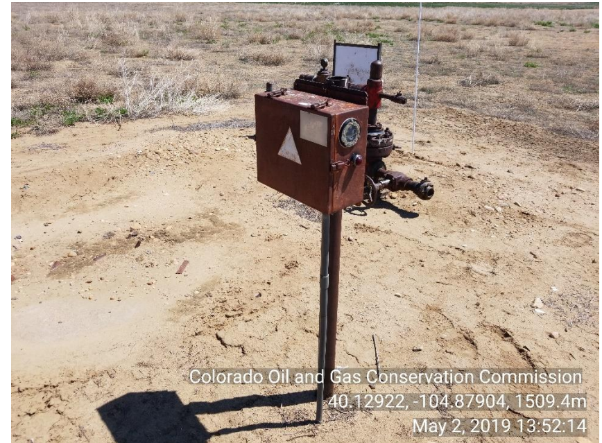
Photo 4 Unused equipment: electric panel.
