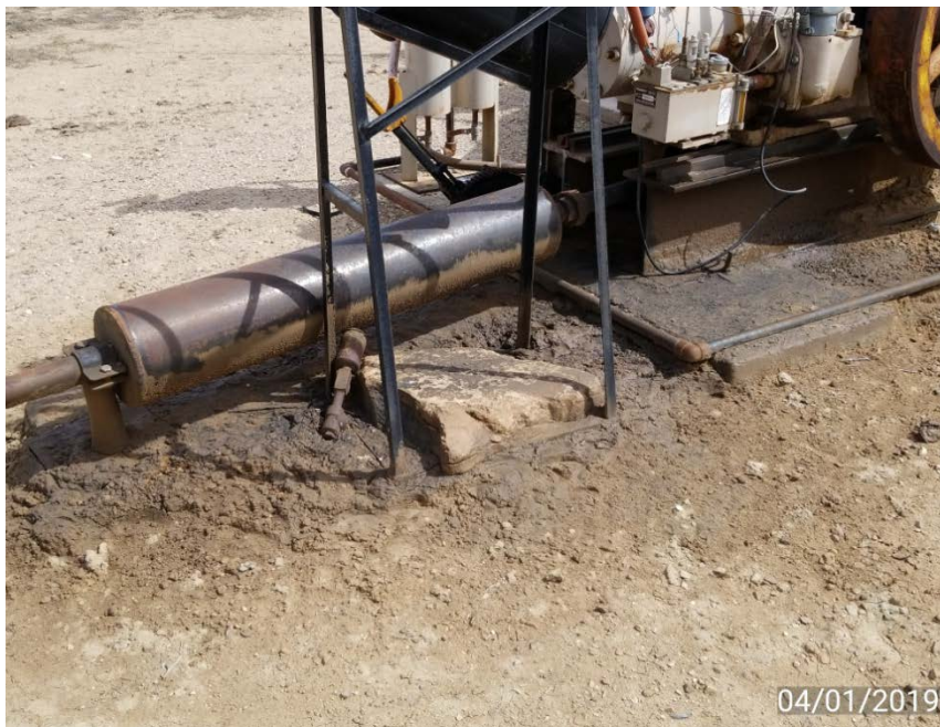
Photo 5. Oily waste on ground at pump jack.
