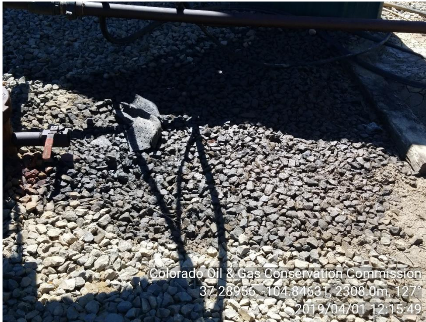
PHOTO 3: STAINED SOIL NEAR WELLHEAD TO THE WEST APP. 5' X 3' OF IMPACTED SOIL.
