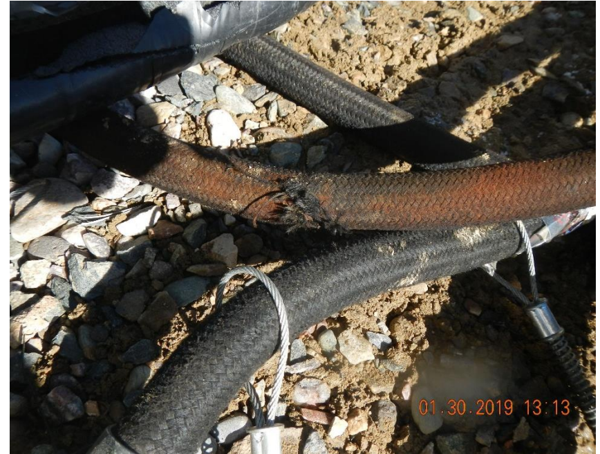
Damaged 1" high pressure hose where release occurred.
