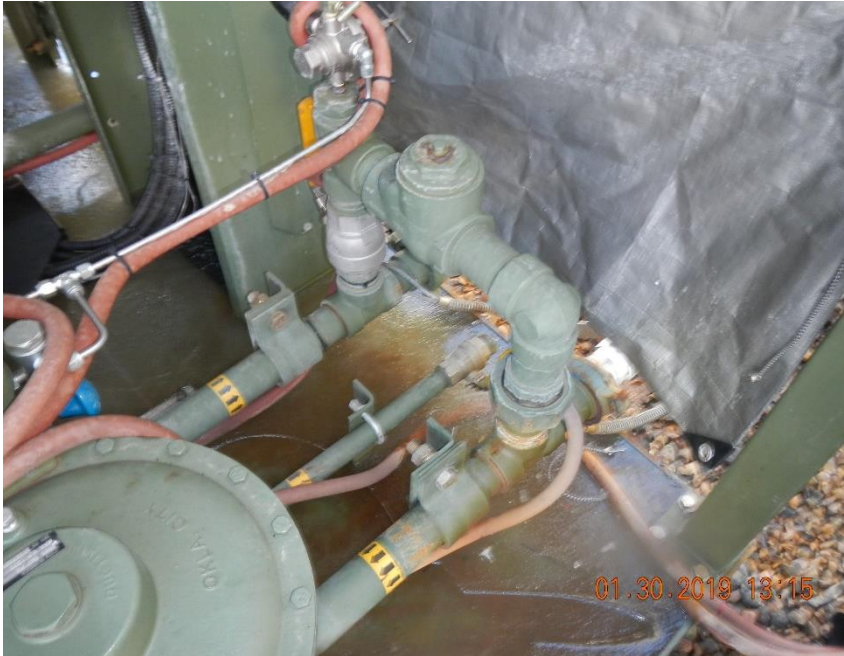
Fitting that failed hose was attached in center of photo.
