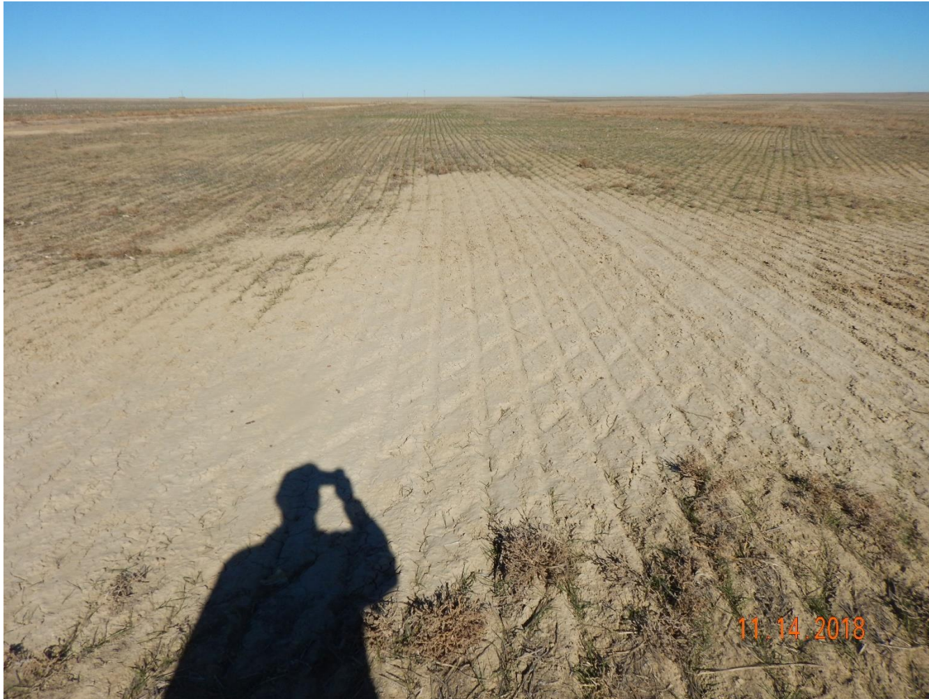
Photo 5: Photo taken from the area of the former battery/pit, facing north. Photo shows area of salt kill down gradient of the pit. Photo shows salt kill remains evident and crop remains unable to establish within these areas.
