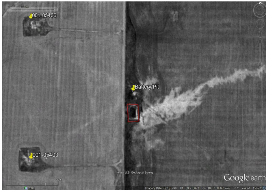
Photo 9: 1998 aerial imagery. Photo shows battery and pit location. Pit in red. Photo also shows a large bare area directly to the east of the well. Bare area likely a salt kill.
