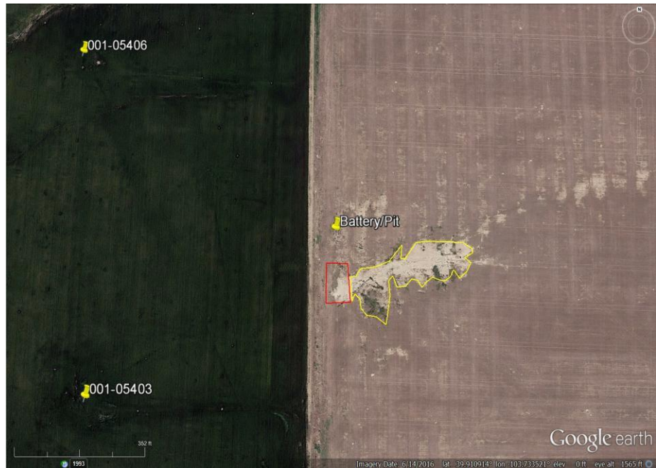
Photo 10: 2016 aerial imagery. Photo shows battery and pit location. Pit in red. Photo also shows a large bare area directly to the east of the well. Bare area likely a salt kill. Main bare area seen in yellow ~1 ac in size.
