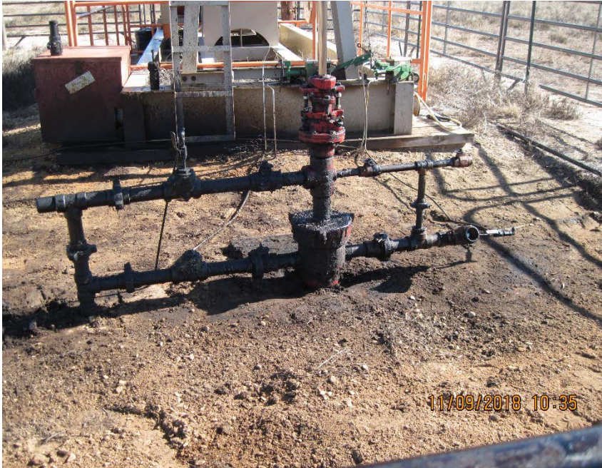
5. Wellhead, after clean up
