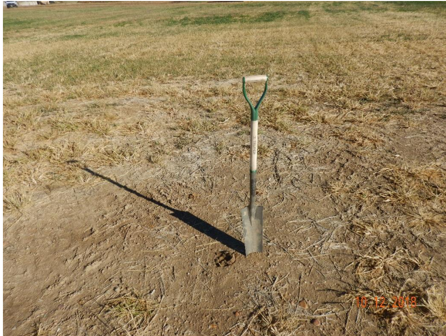
Photo 3: Photo taken from the battery location. Photo shows inspector conducted a compaction test; inspector was only able to easily penetrate the top couple inches of the soil on the location. Compaction concerns remain evident.
