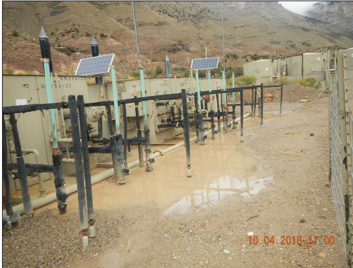
Pooling of storm water at separators.
