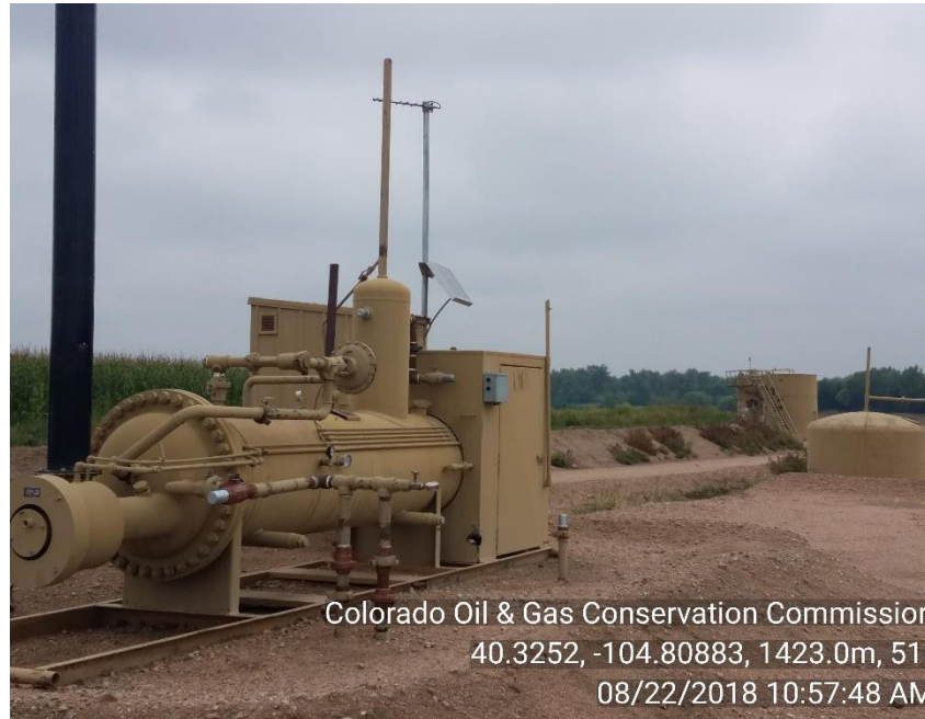
Separator and produce water tank.
