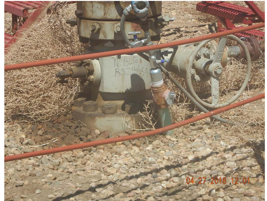
Photo 4: Stained soil at wellhead
