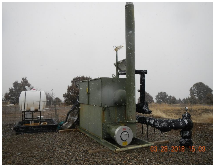
Hotchkiss Federal 1289 #17-11 separator and chemical injection system.
