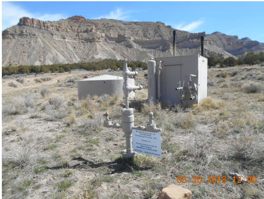
TA wellhead with sign. Unused separator and tank in background.
