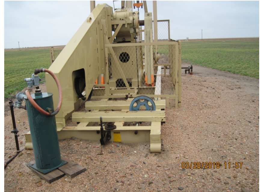
4. Prime mover has been removed
