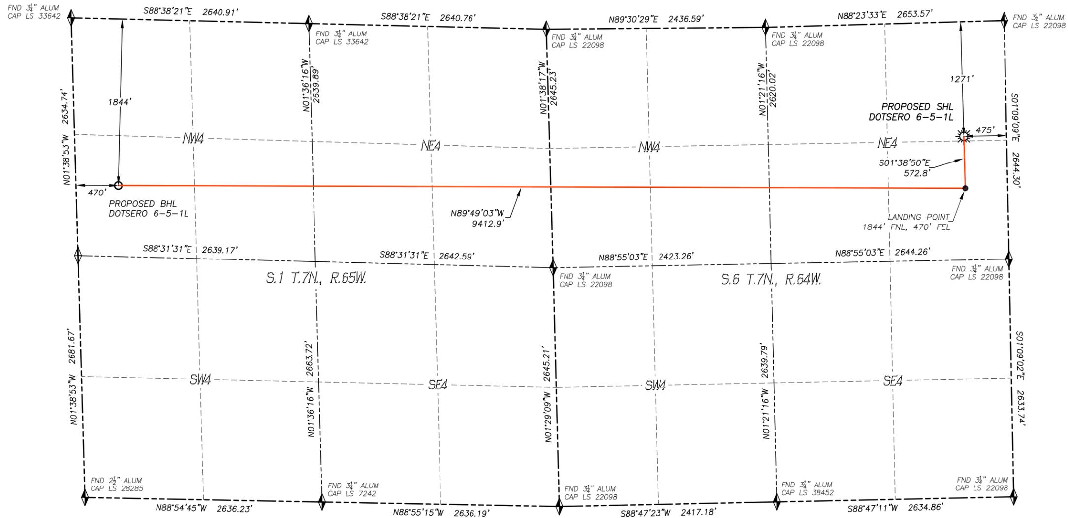
IN ACCORDANCE WITH A REQUEST FROM CONFLUENCE RESOURCES, DALEY LAND SURVEYING, INC. HAS DETERMINED THE SURFACE LOCATION OF THE DOTSERO 6-5-1L WELL TO BE 1271' FNL, 475' FEL, AS MEASURED AT NINETY (90) DEGREES FROM THE SECTION LINES OF SECTION 6, TOWNSHIP 7 NORTH, RANGE 64 WEST, AND THE BOTTOM HOLE LOCATION TO BE 1844' FNL, 470' FWL, AS MEASURED AT NINETY (90) DEGREES FROM THE SECTION LINES OF SECTION 1, TOWNSHIP 7 NORTH, RANGE 65 WEST, OF THE 6TH PRINCIPAL MERIDIAN, WELD COUNTY, COLORADO.
