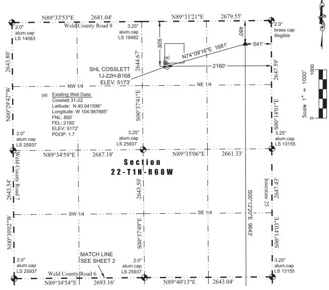
In accordance with a request from Jay Knutson of Crestone Peak Resources, Washburn Land Surveying, LLC has determined the location of the COSSLETT 1J-22H-B168 well site to be SHL: 926' FNL and 2160' FEL, (TPZ: 480' FNL and 541' FEL), (BHL: 460' FSL and 530' FEL), as measured at ninety (90) degrees from the section lines of Sections 22 and 27, Township 1 North, Range 68 West of the 6th Principal Meridian, Weld County Colorado.
