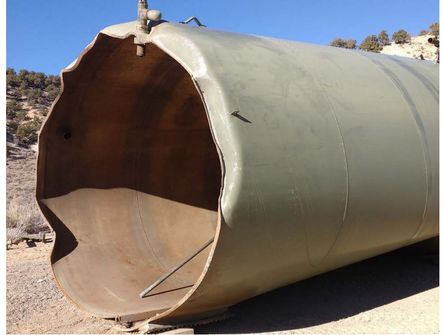
Tank with bottom missing. Tank has been moved from accident area
