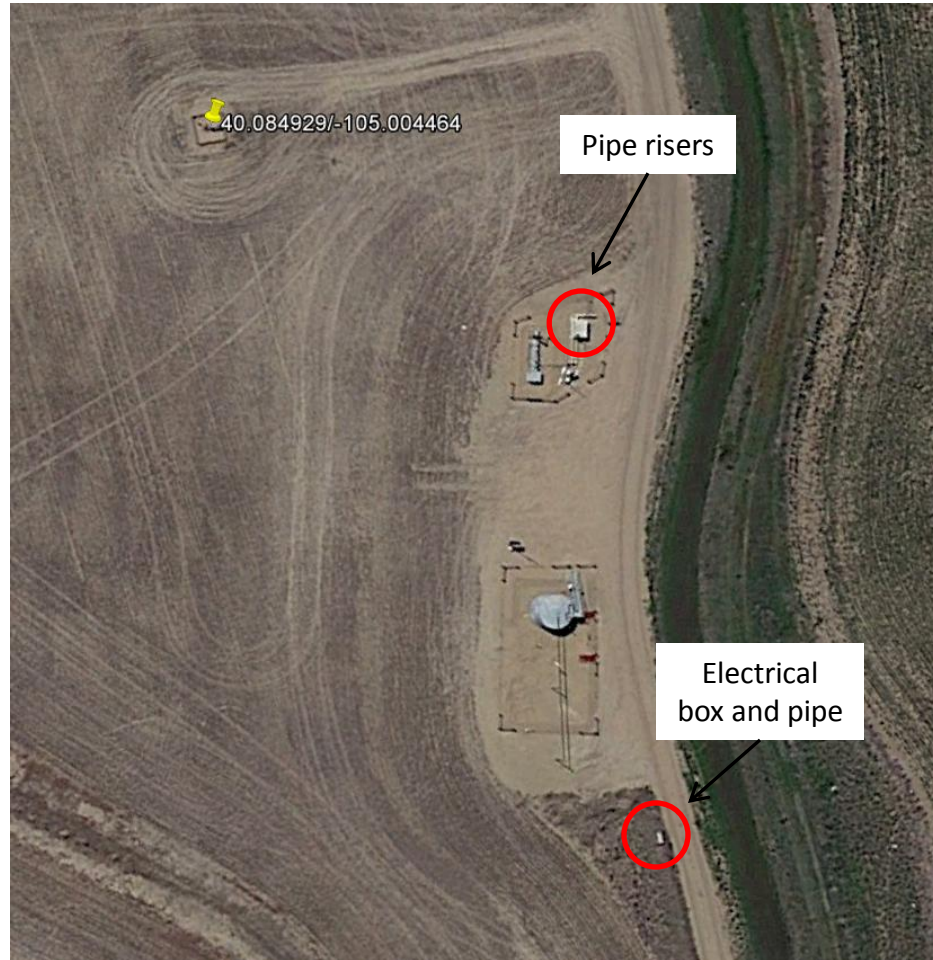
Photo 1. Google Earth aerial imagery taken on June 2, 2014 during active operations. Appears equipment and pipe risers have been left after plugging operations. Well was plugged October 27, 2014.
