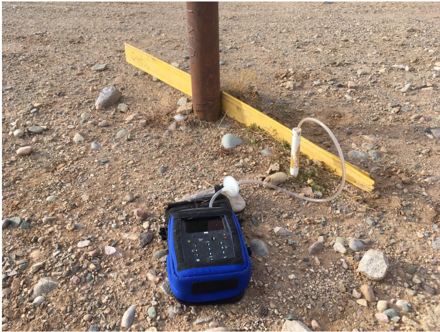
Photo 3. Soil gas measurement instrumentation and soil vapor tube next to plugged and abandoned well marker.
