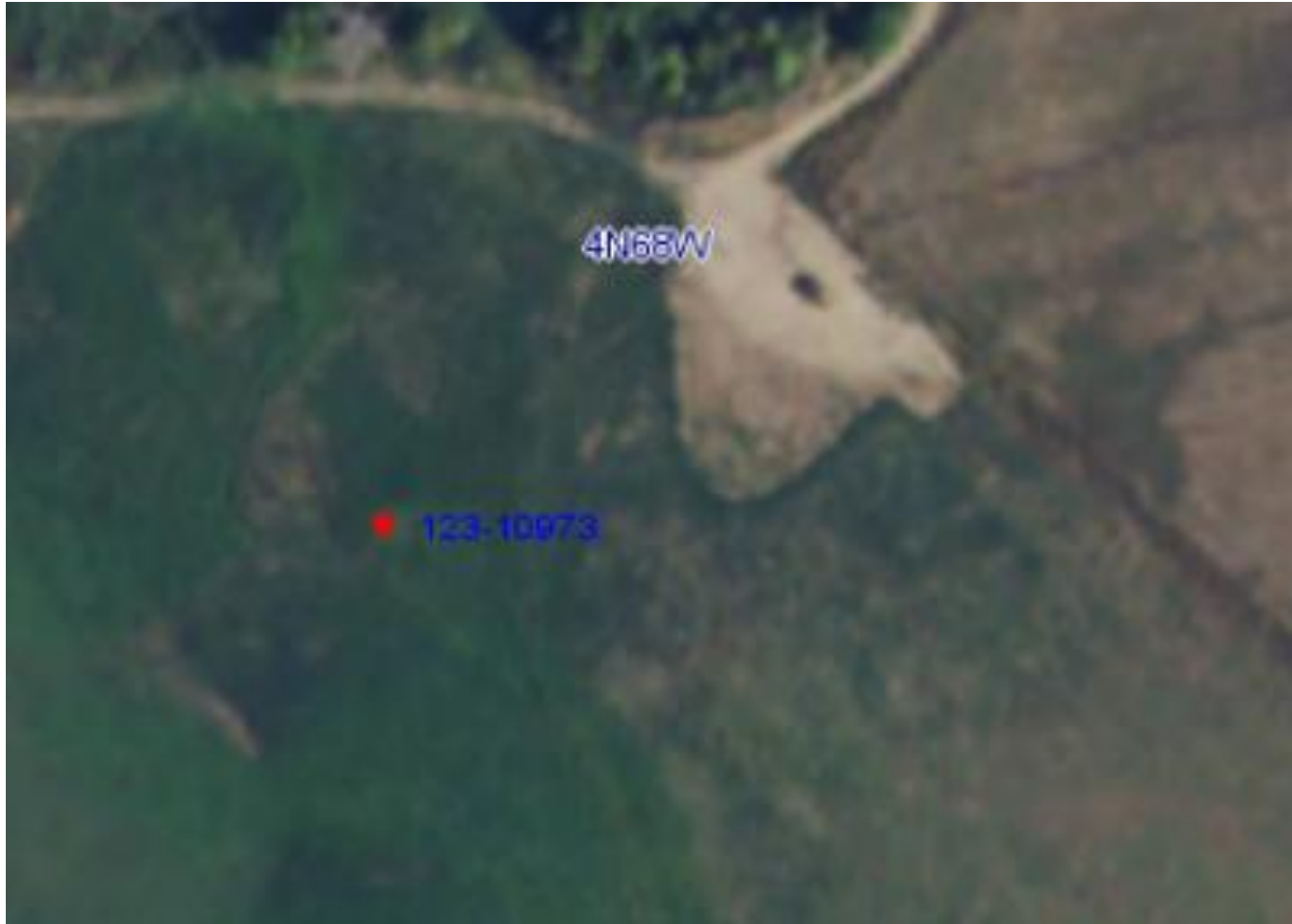
Photo 2. COGCC GISOnline database aerial imagery from 2015 illustrating the well and battery location. The well location appears to meet Rule 1004 standards but the tank battery location does not meet Rule 1004 standards. Refer to the following photos for more detail.
