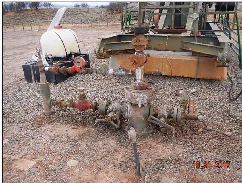
Photo 2. Staining at wellhead.
