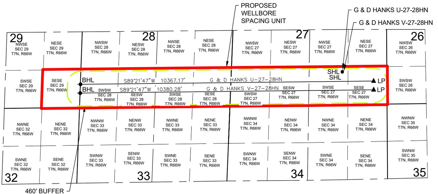
**G & D HANKS U-27-28HN WELL TO BE LOCATED 1183' FSL AND 1575' FEL, SEC 27, T7N, R66W**
