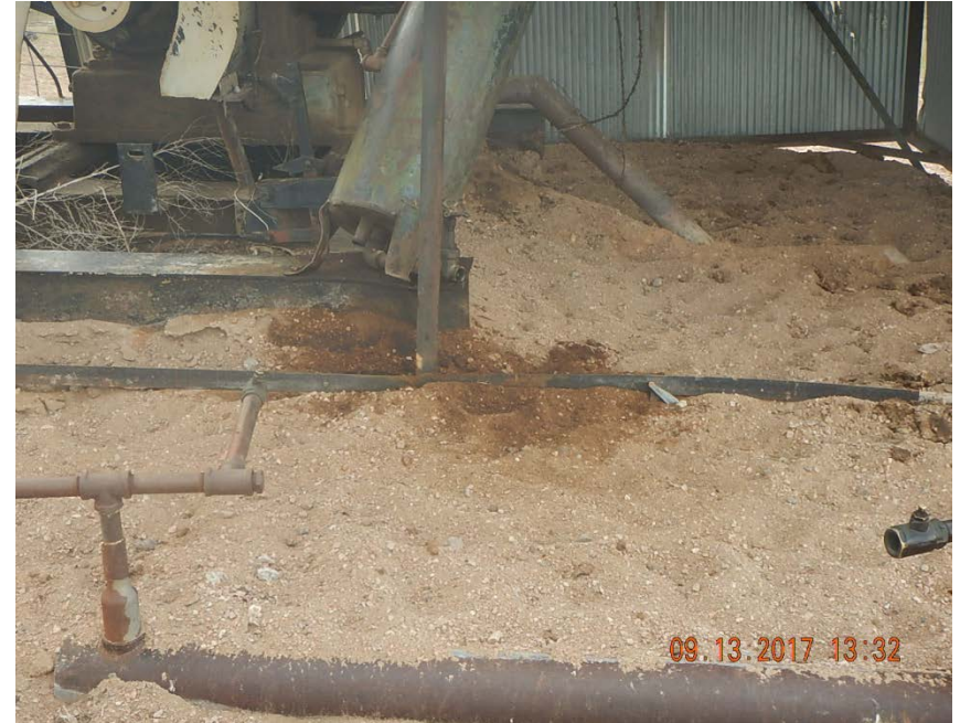
Photo 4: Stained soil at engine
