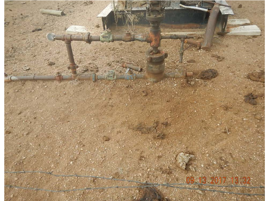
Photo 1: Bradenhead not plumbed to surface.
