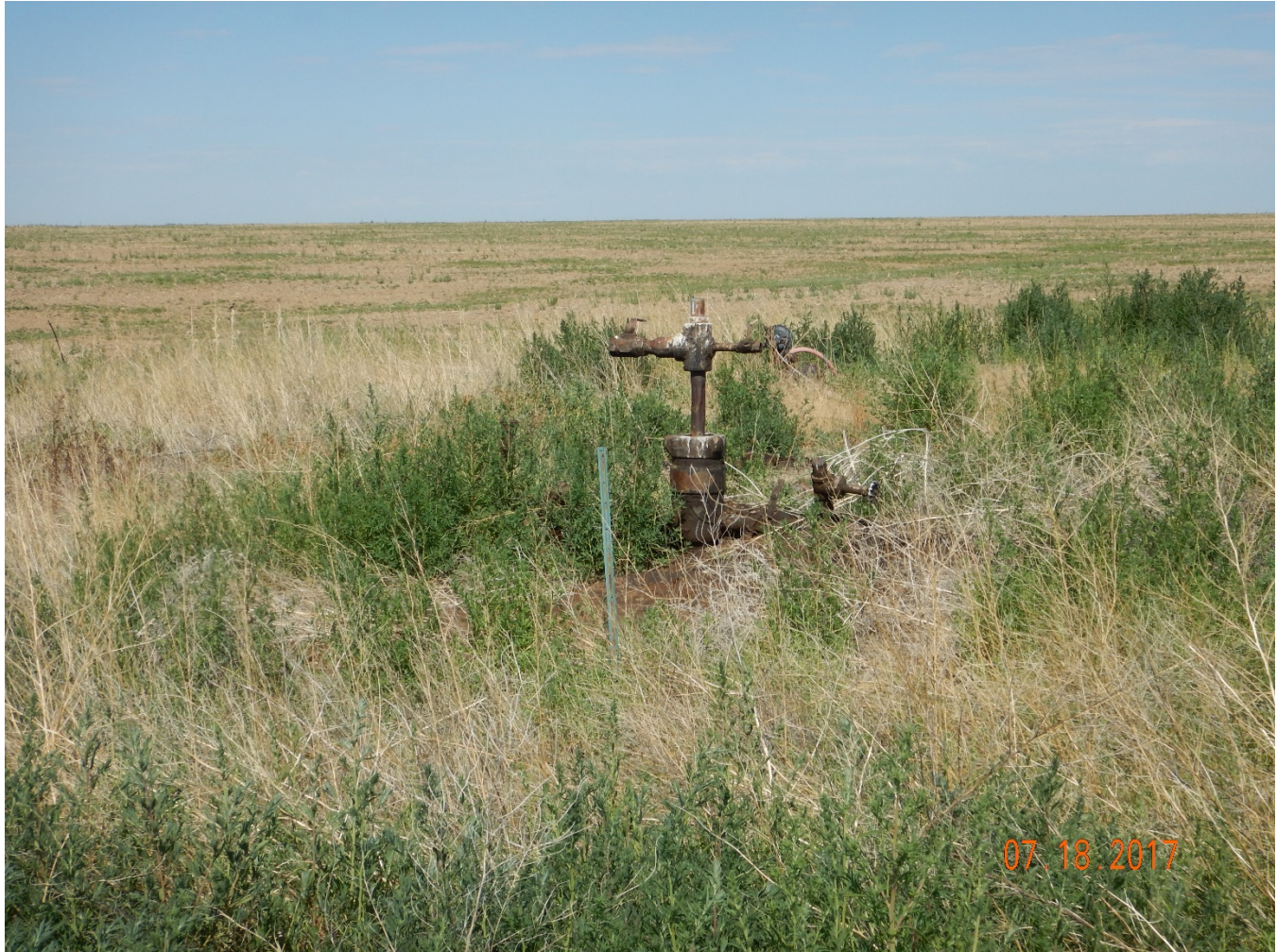
Photo 9 - Significant accumulation of oily waste localized at wellhead. Note absence of wellhead sign.
