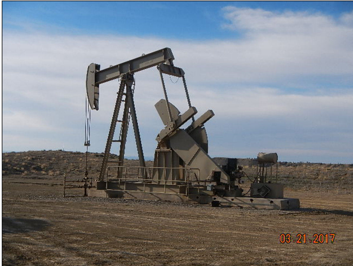
Photo 1. Pump jack and wellhead.
