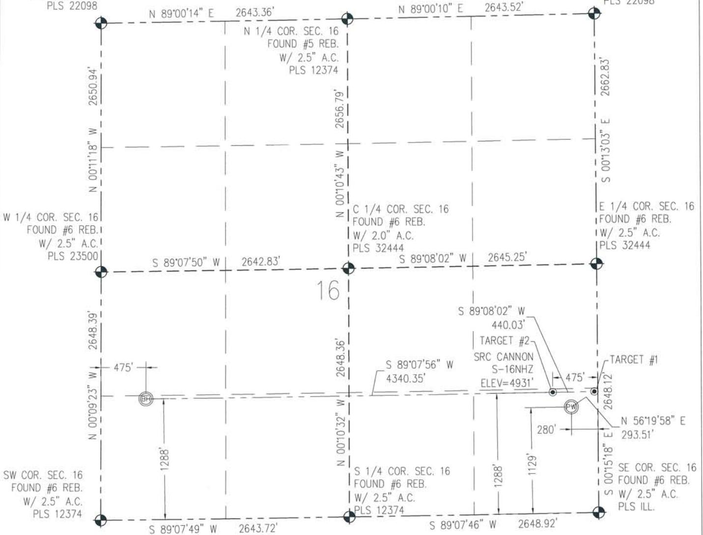
**N** IN ACCORDANCE WITH A REQUEST FROM CRAIG RASMUSON - SYNERGY RESOURCES, BASELINE ENGINEERING CORP. HAS DETERMINED THE LOCATION OF THE SRC CANNON S-16NHZ TO BE 1129' FSL AND 280' FEL, AS MEASURED AT NINETY (90) DEGREES FROM THE SECTION LINE OF SECTION 16, TOWNSHIP 4 NORTH, RANGE 68 WEST AND THE BOTTOM HOLE LOCATION TO BE 1288' FSL AND 475' FWL OF SECTION 16, TOWNSHIP 4 NORTH, RANGE 68 WEST, 6TH PRINCIPAL MERIDIAN, WELD COUNTY, COLORADO.
