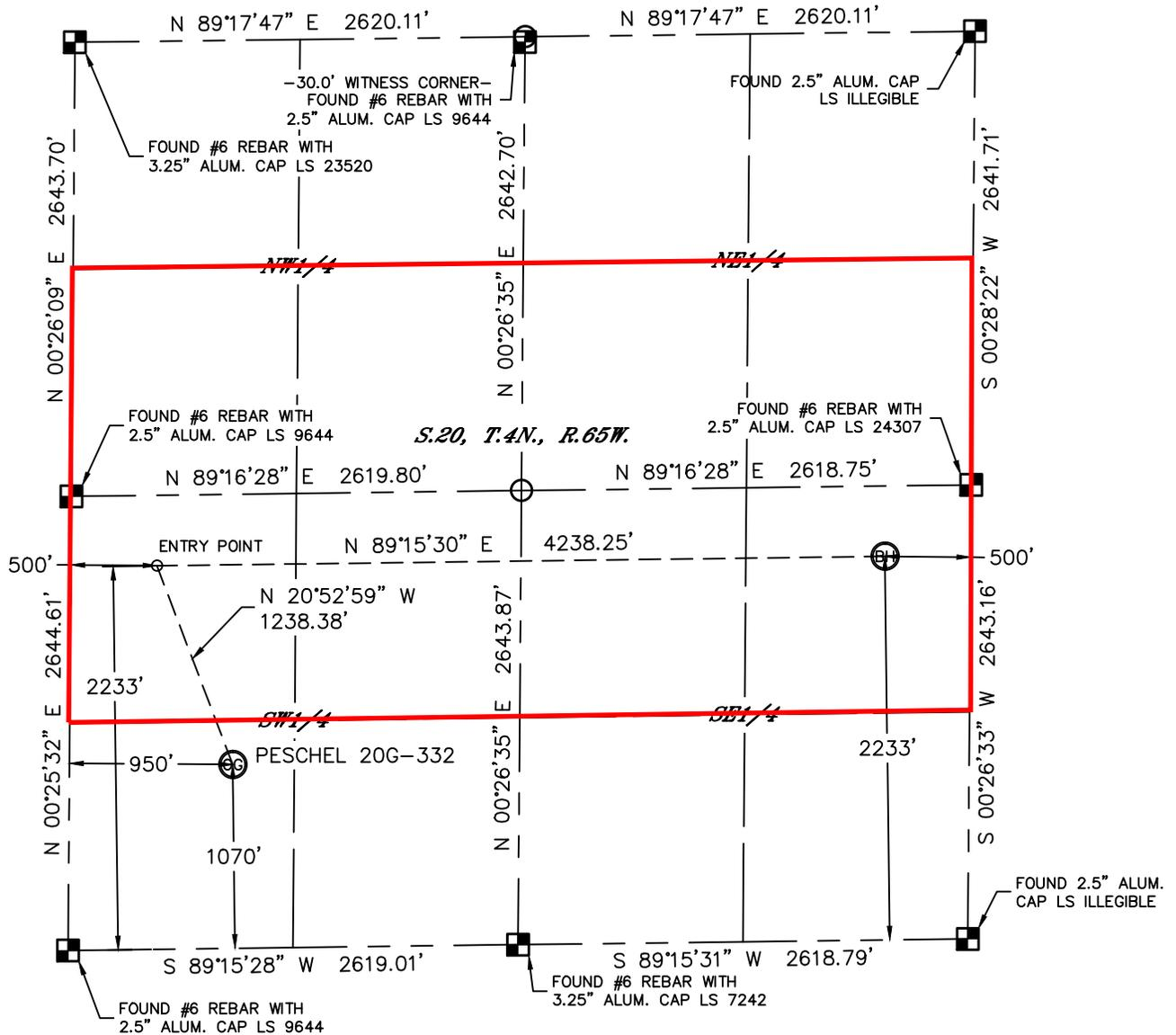
In accordance with a request from Jake Bragg with PDC ENERGY Lat40°, Inc. has determined the surface location of the PESCHEL 20G-332 to be 1070' from the SOUTH line and 950' from the WEST line and the bottom hole to be 2233' from the SOUTH line and 500' from the EAST line as measured at right angles from the section lines of Section 20, Township 4 North, Range 65 West of the Sixth Principal Meridian, County of Weld, State of Colorado.
