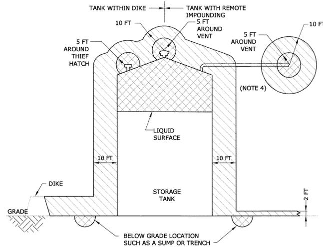
NOTE 1 HIGH FILLING RATES OR BLENDING OPERATIONS INVOLVING CLASS I FLAMMABLE LIQUIDS MAY REQUIRE EXTENDING THE BOUNDARIES OF CLASSIFIED AREAS.
